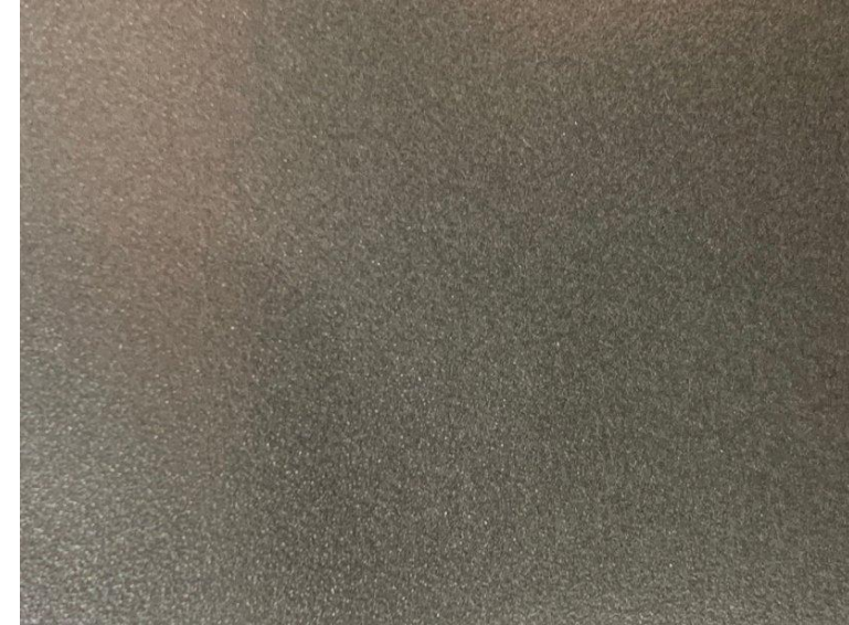
Enlarged Image of Matte Embossed Film with 3µm Depth
